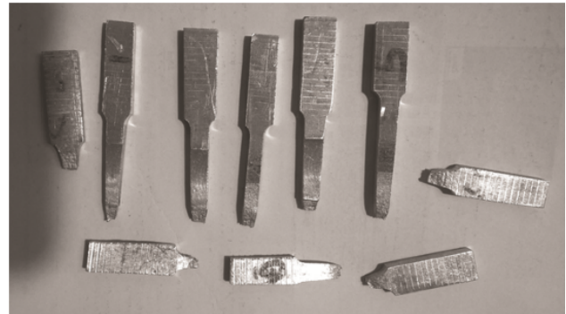
Figure 4: Transverse tensile specimen
